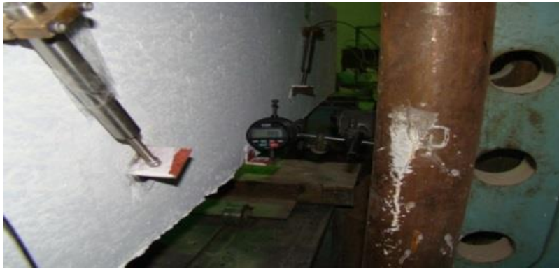
Fig.1 : Deflection digital dial gauge at mid-span of beams.
